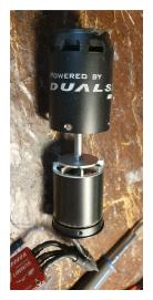
The motor is designed just like the other canned Dualsky motors as an outrunner that is encapsuled so that the wires can come out from the back and the motor can be screwed directly to the bulkhead. I must say it is amazing quality and the motor never touch the outer shell even at much higher loads than intended on the design.
